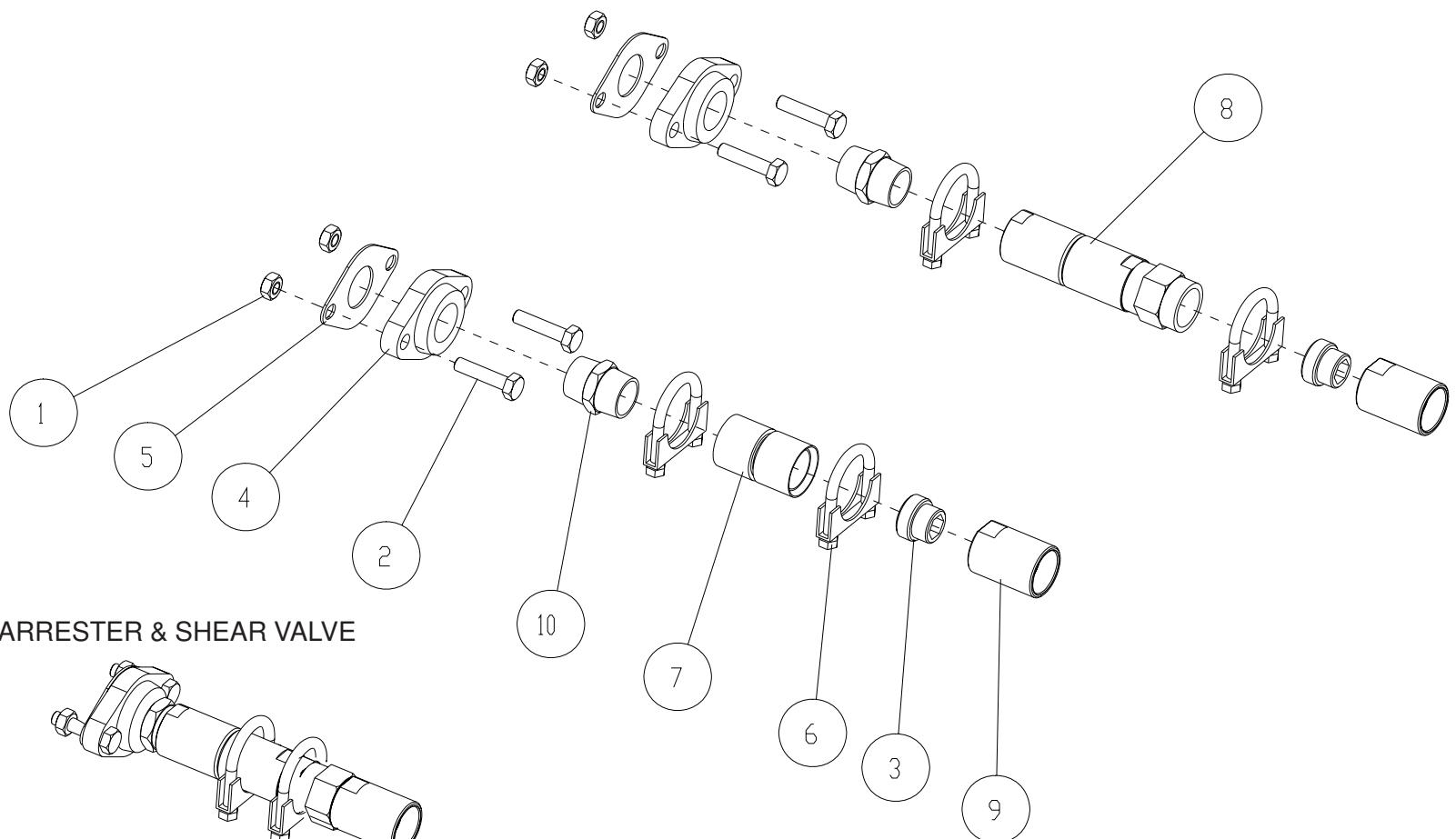
VR FLAME ARRESTER & SHEAR VALVE
